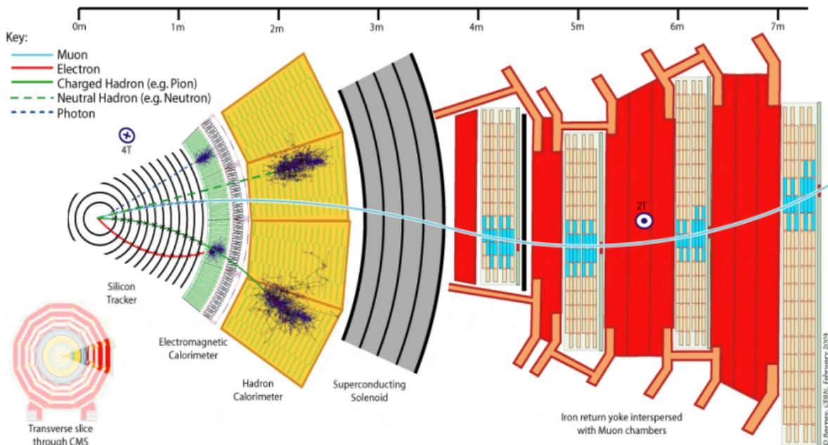
Reconstruction makes use of the muon chambers and the silicon tracker by first finding a segment in the muon stations (StandAlone Muons), which is then matched to a compatible track in the silicon tracker (Tracker tracks). A combined fit of the muon segment and silicon tracks trajectory yields the final reconstructed muon track (Global Muons). The  $\eta$ -coverage for muon reconstruction in the CMS detector is  $|\eta| < 2.4$ .
