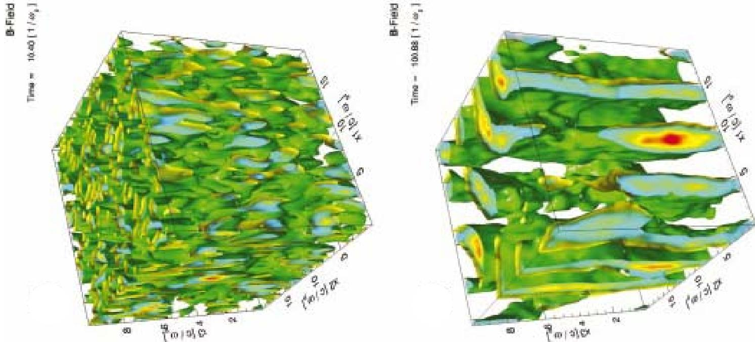
Magnetic field energy density for values of 15% of the maximum energy density. Results are shown slightly before saturation and in the quasi-static stage ( $\epsilon_B \sim 1\%$ ).
